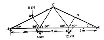
Determine the nature and magnitude of the forces in the members BC. GC and GF of the truss
